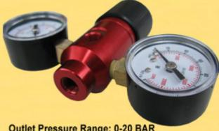
Outlet Pressure Range: 0-20 BAR Maximum Inlet Pressure: 150 BAR Safety Relief Valve: 25 BAR Outlet Connection: 1/8" Gas
